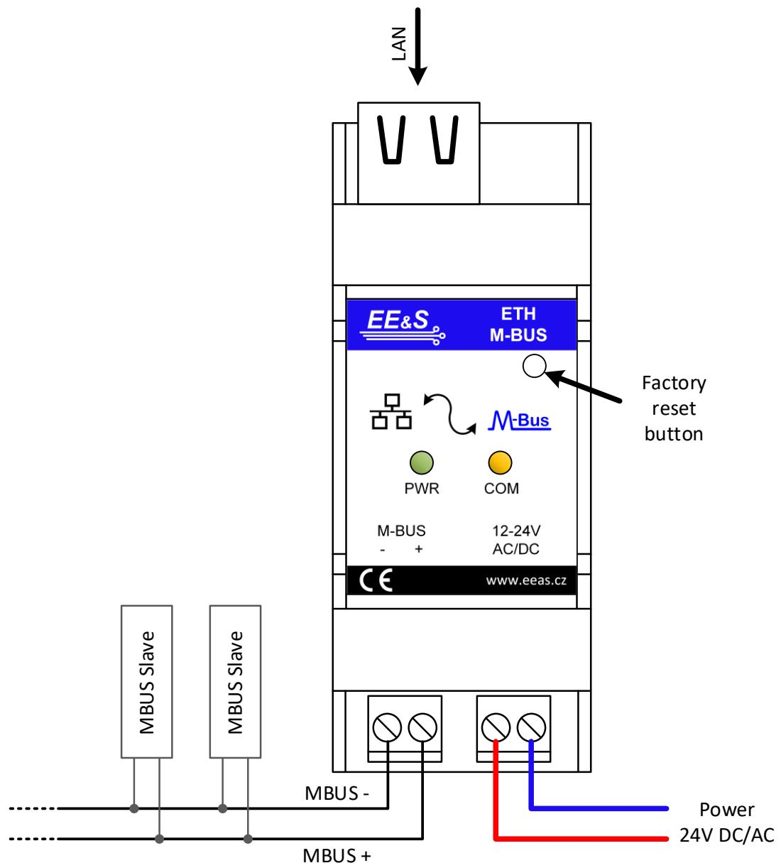
The device is equipped with two LEDs. The green LED labeled as "PWR" indicates the presence of the power supply with a steady light. The yellow LED labeled as "COM" flashes when a packet is sent to or received from the MBUS line. In addition there is a factory reset button on the right top part.
