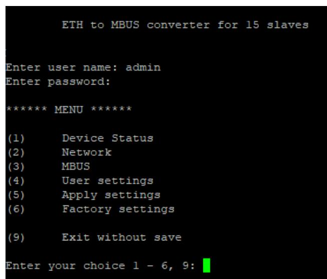
The telnet interface will guide you through selected settings. For instance, setting the MBUS interface (menu “3”) flow looks like. The value shown in brackets remains unchanged if the user just presses Enter without typing a new value.
